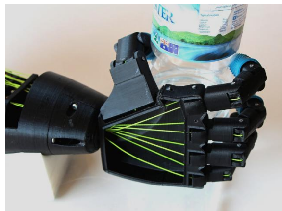
Figure 8. Bionic hand holding an object
