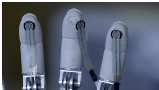
Figure 9: Force sensors placed at fingers' end
