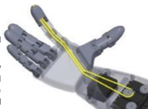
Figure 35: Moving a finger of the bionic hand
